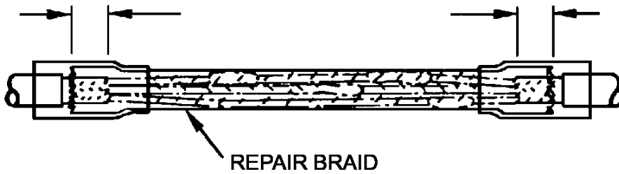
Figure 15. Repair Braid Centered Over Repair Area.
